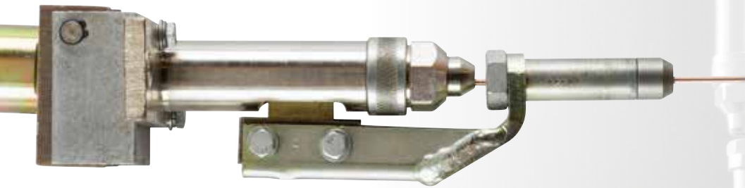
Positive Contact torch and its extension providing Long Stick Out (125 mm)
