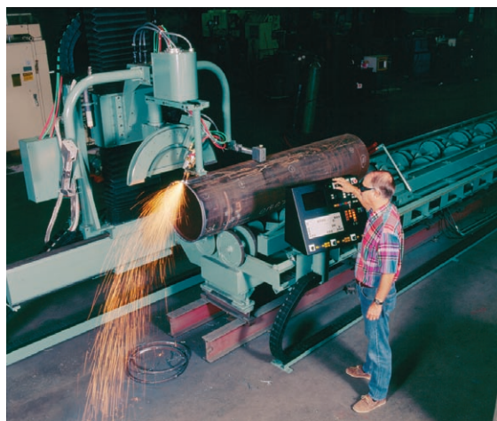
Figure 2. Mechanism of cutting improves the speed and repeatability of each contour. All cutting operations are controlled by one person from the operator console.
