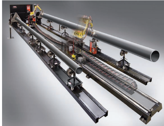
Figure 1. Fully automated robotic pipe welding system with horizontal travel carriage.
