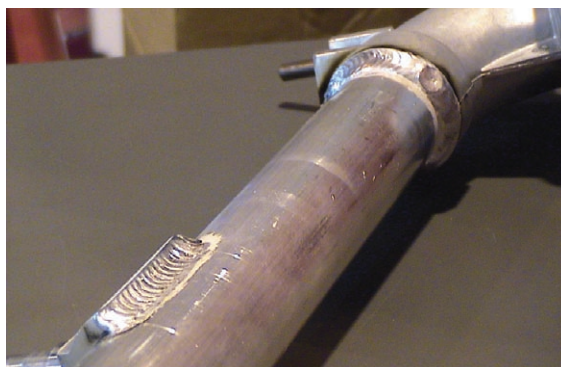
Figure 6. Aluminium pipe can be welded using an extended-land joint geometry. Uniform aluminium weld bead using MIG Welding that approaches the level of quality, appearance and integrity commonly associated with TIG welding.
