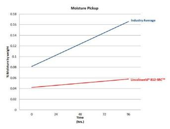
**Figure 5.** Low initial moisture and low moisture pick up provide low risk of delayed cracking.
