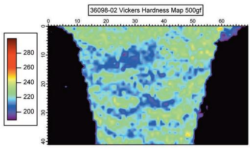
Figure 2. Weld metal hardness is reduced by heat treatment (mapped with approximately 2000 indentations).
