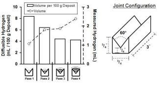
Figure 4. Diffusible hydrogen in various layers of multiple-pass welds.
