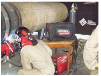
**Figure 4.** The welding team combined an orbital pipe welder, the Dyna Torque LONESTAR Automated Welding System, with Lincoln Electric's innovative Pipeliner® 80Ni1, a gas metal arc welding (GMAW) wire developed specifically for the global pipe welding industry.
