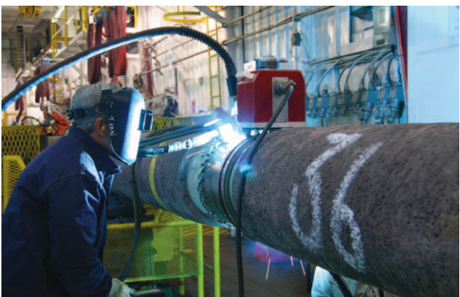
Figure 3. McDermott's JBBS welding system.
