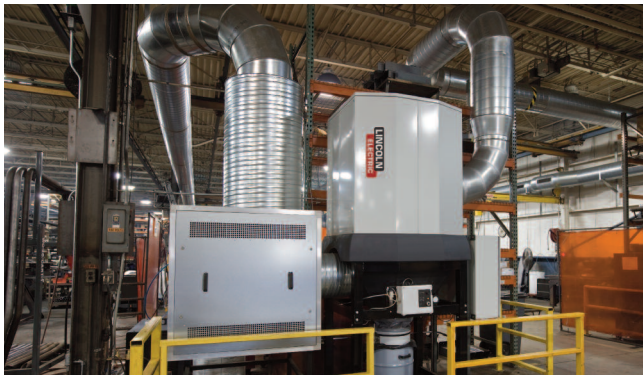
The fan and self-cleaning filtration units were selected specifically for Elgin's push/pull system.
