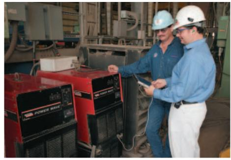
Wave AC/DC, polarities and waveshapes can be changed via software on the fly with a much greater degree of control, allowing the welder to optimize the penetration profile while maintaining the highest possible deposition rate.
